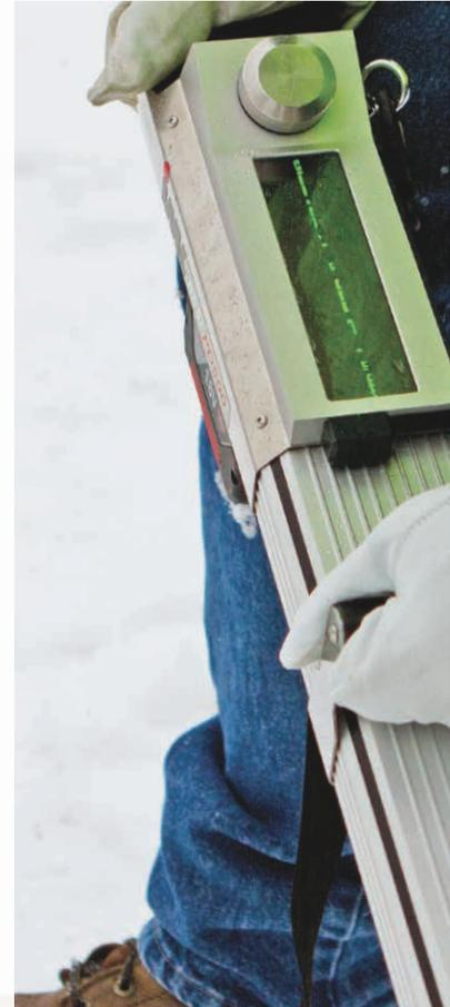
*The PD500 Resistograph allows the user to identify soft spots and voids inside the wood to determine a utility pole's strength.*
